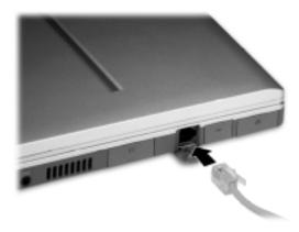
**4.** Connect the other end of the RJ-11 telephone cable into an (analog) phone jack.
